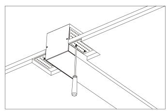
4. Place the profile into the cut-out hole with the L brackets fitting into the small recess made area. Secure L brackets accordingly.
