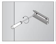
1. Attach the wall side clip to surface
