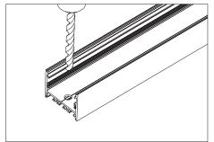
1.Drill a hole on the aluminium
