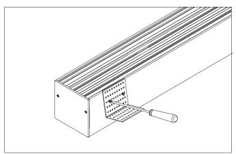
3. Screw on the perforated L brackets to the profile
