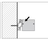
3. Mount the light fixture onto the wall attachment
